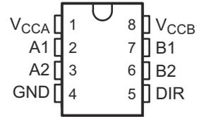
Figure 4-1. DCU Package, 5-Pin VSSOP (Top View)
