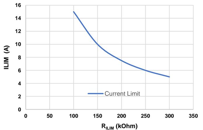
Figure 6. Inductor Peak Current Limit vs RLIM Resistance
