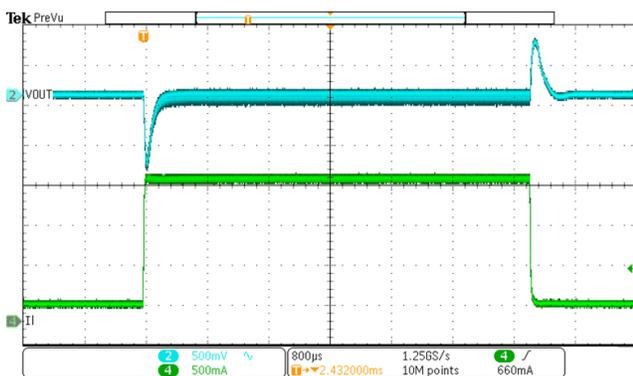
Figure 19. Load Transient (Vout=15V, Iout=0.2A to 1.8A, SR=250mA/us)
