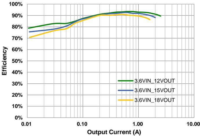
Figure 3. Efficiency, fsw=400 kHz, 1-cell Battery, PFM
