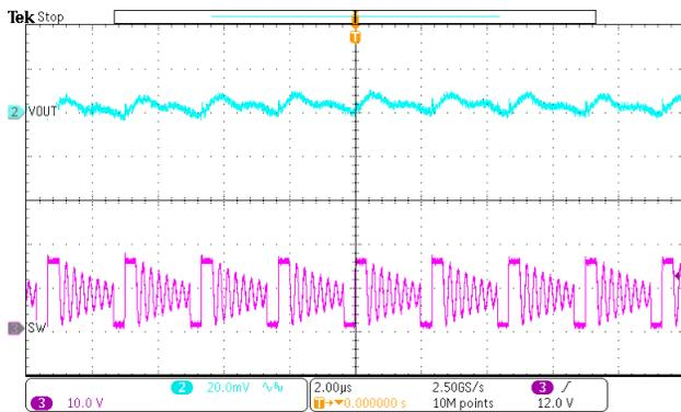
Figure 15. Switching Waveforms and Output Ripple (Vout=15V, Iout=100mA)
