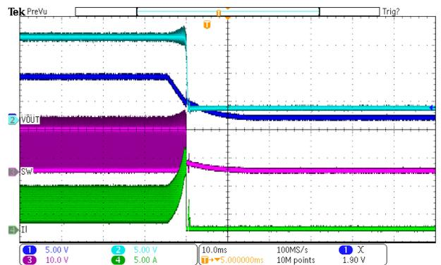
Figure 18. Power Down (Vout=15V, Iout=2A)
