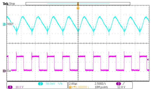
Figure 16. Switching Waveforms and Output Ripple (Vout=15V, Iout=2A)
