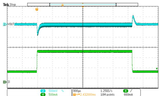
Figure 20. Load Transient (Vout=15V, Iout=0.5A to 1.5A, SR=250mA/us)
