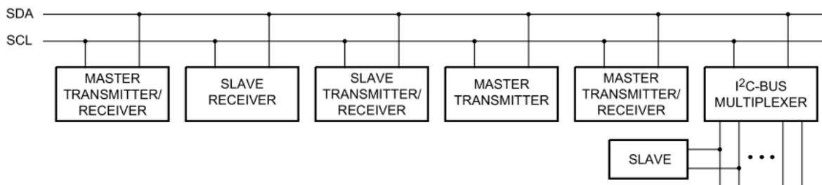
**Figure 9. System Configuration**
