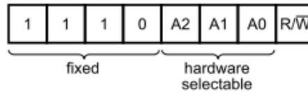
**Figure 4. Device Address**
