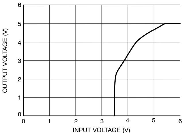
Figure 13. Output Voltage vs. Input Voltage, 5 mA Load
