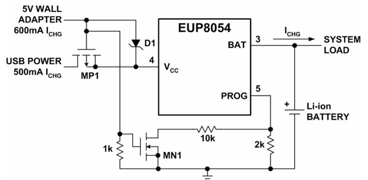
**Figure 12. Combining Wall Adapter and USB Power**
