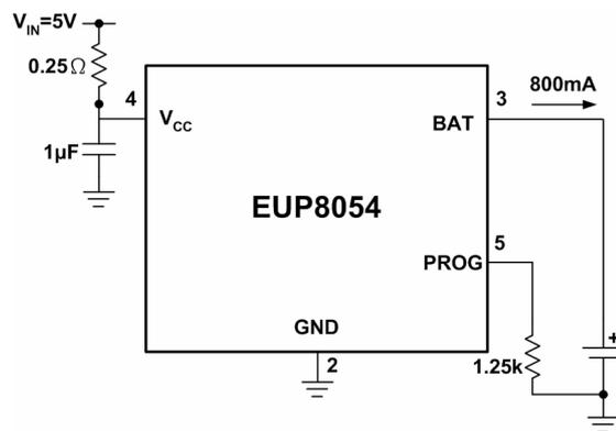
Figure 4. 800mA Li-Ion Charger with External Power Dissipation
