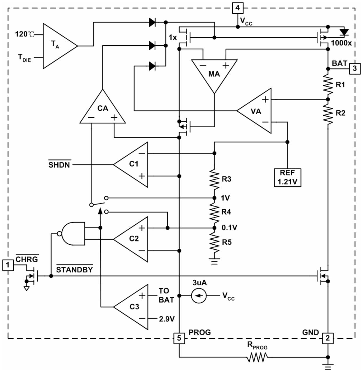
Figure 6. Block Diagram
