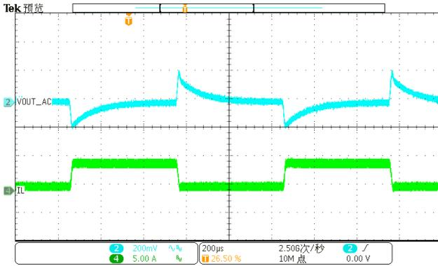
Figure 19. Load Transient (0.5A-4.5A, 1.6A/us)
