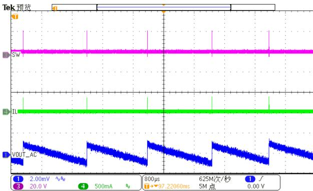
Figure 21. Output Ripple (Iload=0A)
