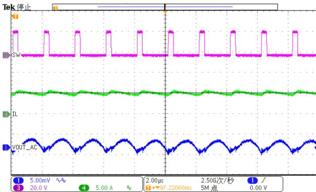
Figure 23. Output Ripple (Iload=5A)
