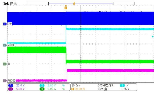
Figure 18. Over Current Release (hard short to 1A)
