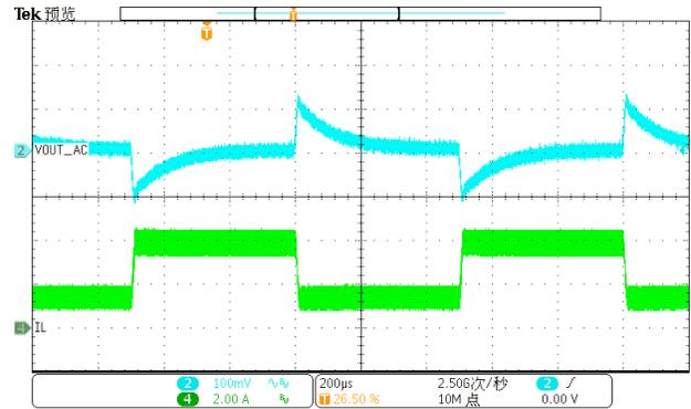
Figure 20. Load Transient (1.25A-3.75A, 1.6A/us)
