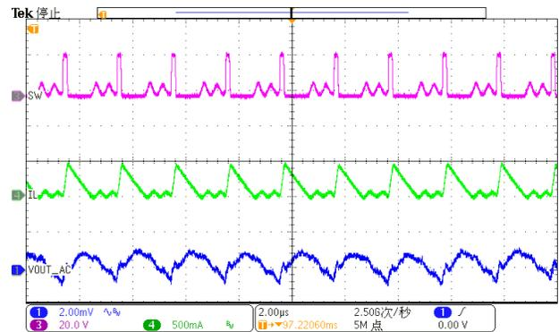
Figure 22. Output Ripple (Iload=100mA)
