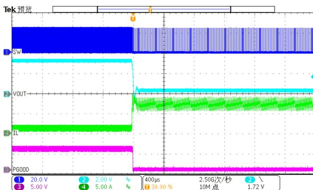
Figure 17. Over Current Protection(1A to hard short)
