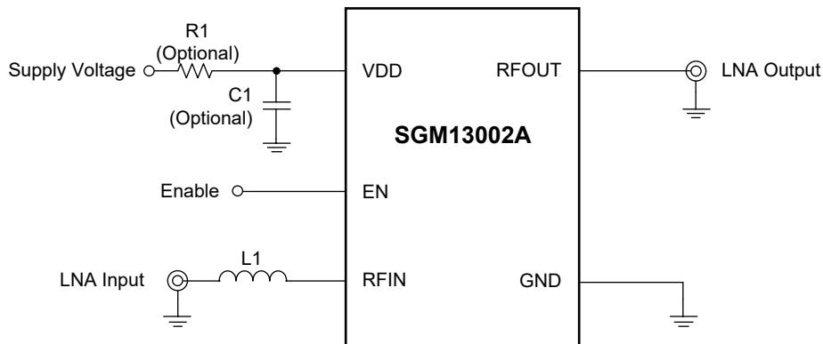
Figure 2. SGM13002A Typical Application Circuit
