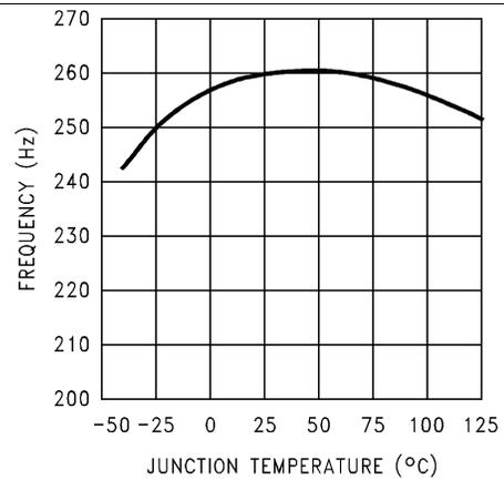
Figure 10. Switching Frequency
