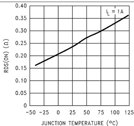
Figure 4. Drain-to-Source Resistance
