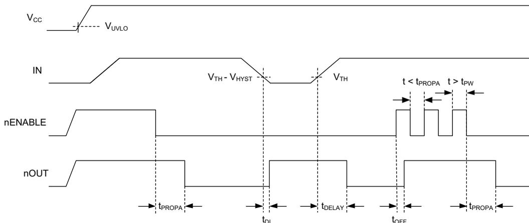
**Figure 5. SGM896A/SGM898A Timing Diagram**
