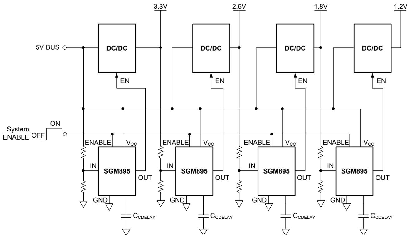
Figure 11. Multiple-Output Sequencing
