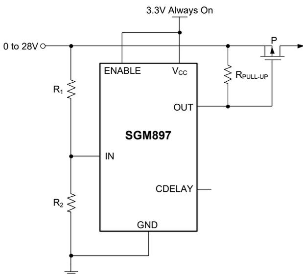
**Figure 9. Over-Voltage Protection**
