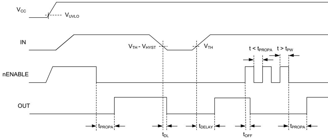
**Figure 7. SGM899A Timing Diagram**
