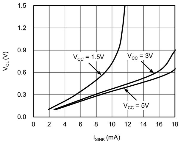
Output Low Voltage vs. Sink Current
