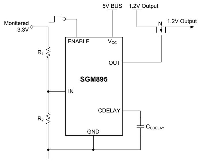
**Figure 10. Low-Voltage Sequencing Using an N-Channel MOSFET**
