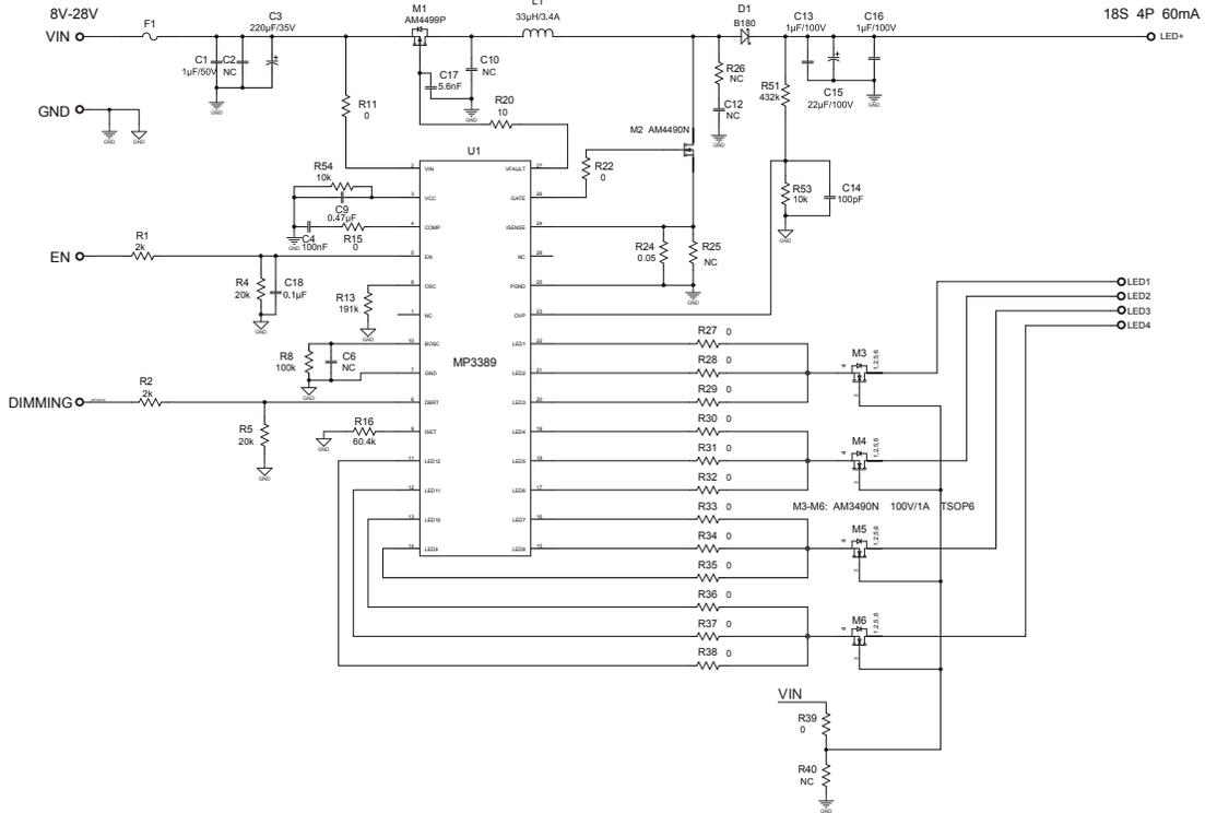
Figure 8 – Drive 18LEDs in Series, 4 strings 60mA/string
