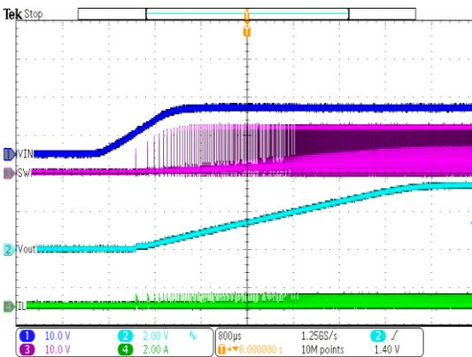
Figure 13. Power Up, Iout=10mA
