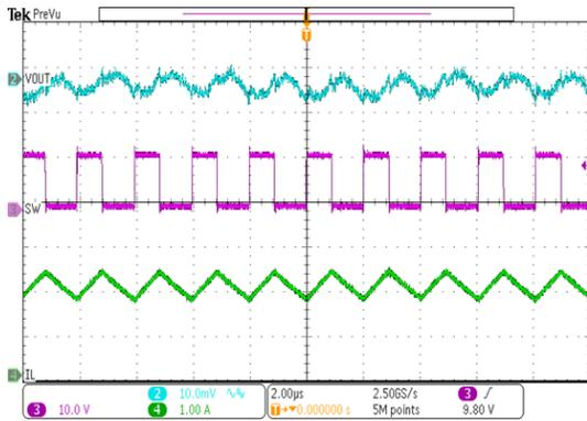
Figure 11. SW node waveform and Output Ripple, Iout=2A
