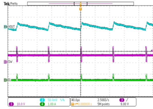
Figure 12. SW node Waveform and Output Ripple, Iout=10mA
