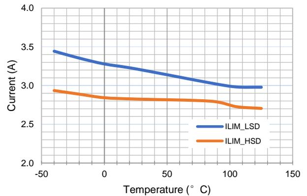
Figure 6. Peak Current Limit vs Temperature
