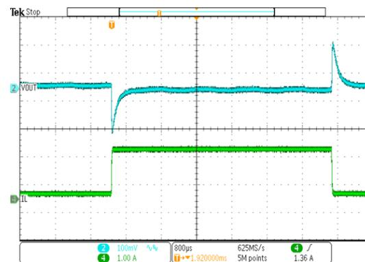
Figure 15. Load Transient (Vout=5V, Iout=0.2A to 1.8A, SR=250mA/us)
