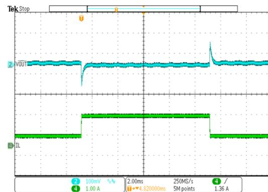
Figure 16. Load Transient (Vout=5V, Iout=0.5A to 1.5A, SR=250mA/us)
