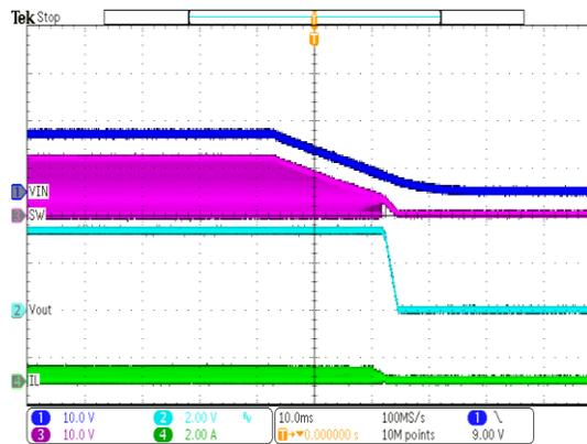
Figure 14. Power Down, Iout=10mA
