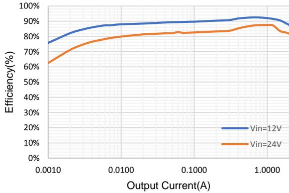
Figure 1. Efficiency, Vout=3.3V
