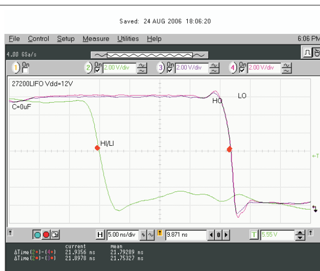
Figure 31. V_{LO} and V_{HO} Falling Edge Delay Matching
