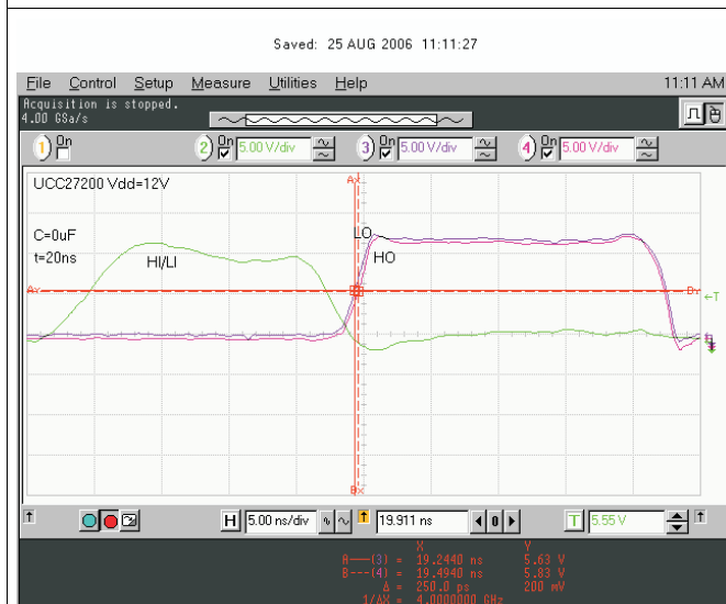
Figure 32. 20-ns Input Pulse Delay Matching
