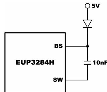
**Figure 4. Add Optional External Bootstrap Diode to Enhance**
