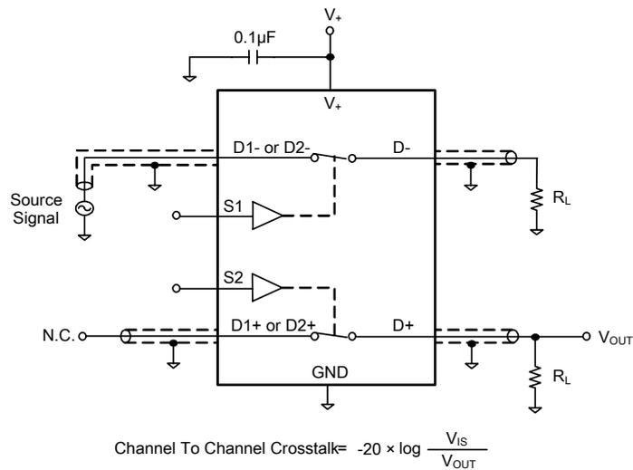
Test Circuit 6. Channel-to-Channel Crosstalk
