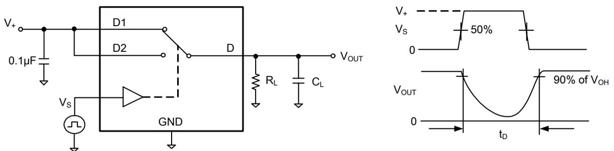
Test Circuit 3. Break-Before-Make Time Delay ( $t_D$ )
