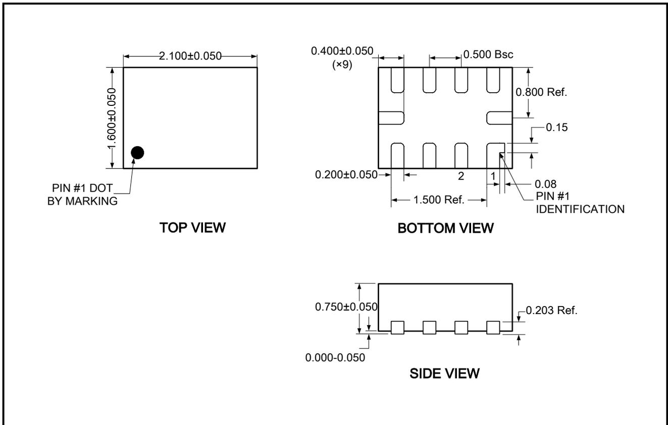
Note: All linear dimensions are in millimeters.
