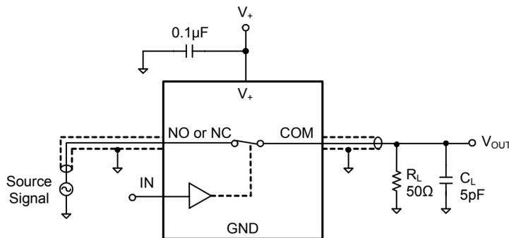
Test Circuit 8. -3dB Bandwidth
