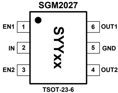
NOTE: The location of pin 1 on the SGM2027 is determined by orienting the package marking as shown.
