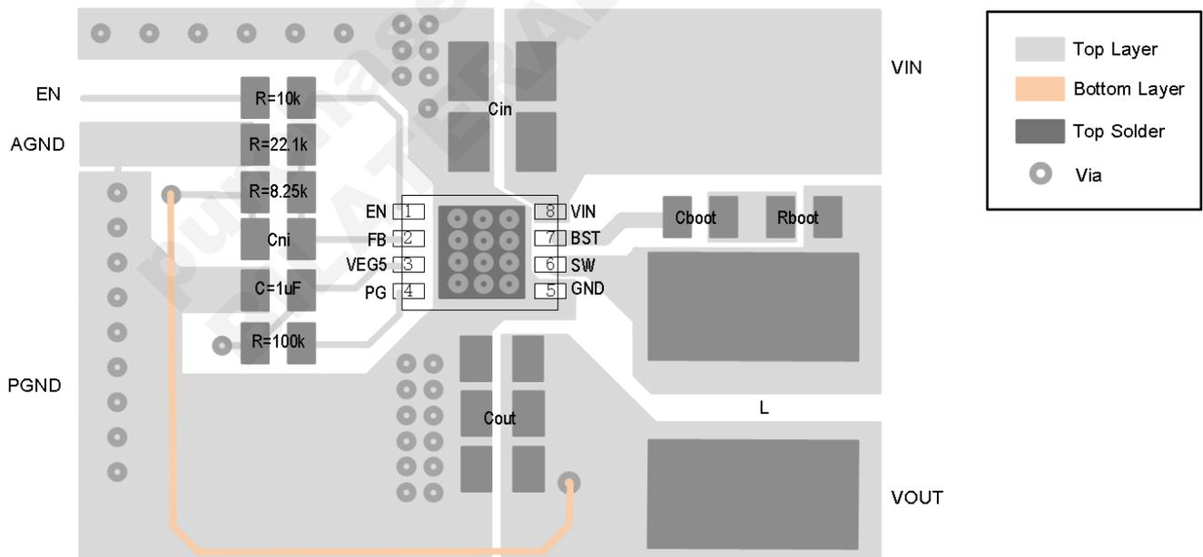
Figure 4. PCB Layout
