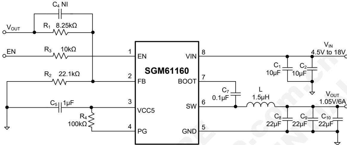
Figure 3. 1.05V/6A Power Supply Design Example with SGM61160
