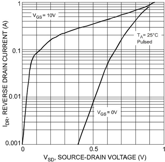
Fig. 9 Reverse Drain Current vs. Source-Drain Voltage
