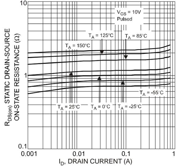
Fig. 4 Static Drain-Source On-Resistance vs. Drain Current
