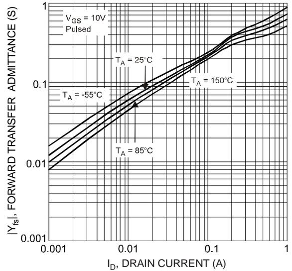
Fig. 10 Forward Transfer Admittance vs. Drain Current
