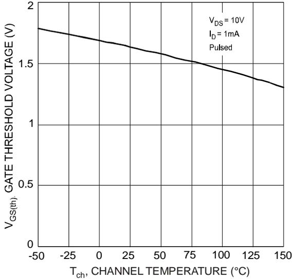
Fig. 3 Gate Threshold Voltage vs. Channel Temperature
