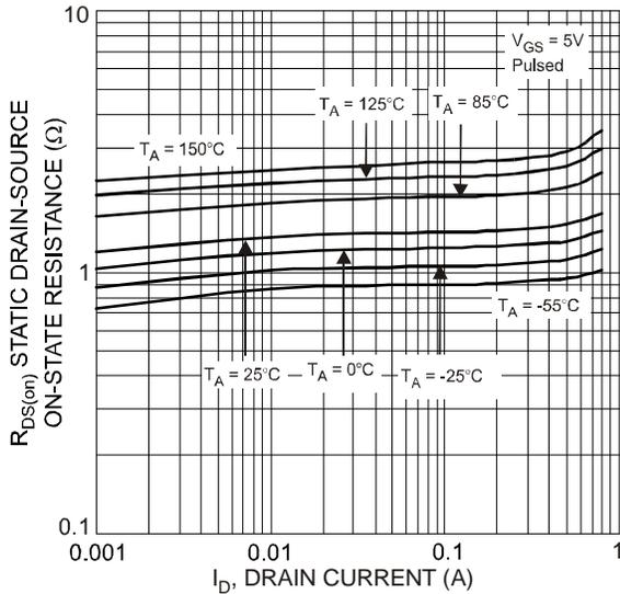
Fig. 5 Static Drain-Source On-Resistance vs. Drain Current
